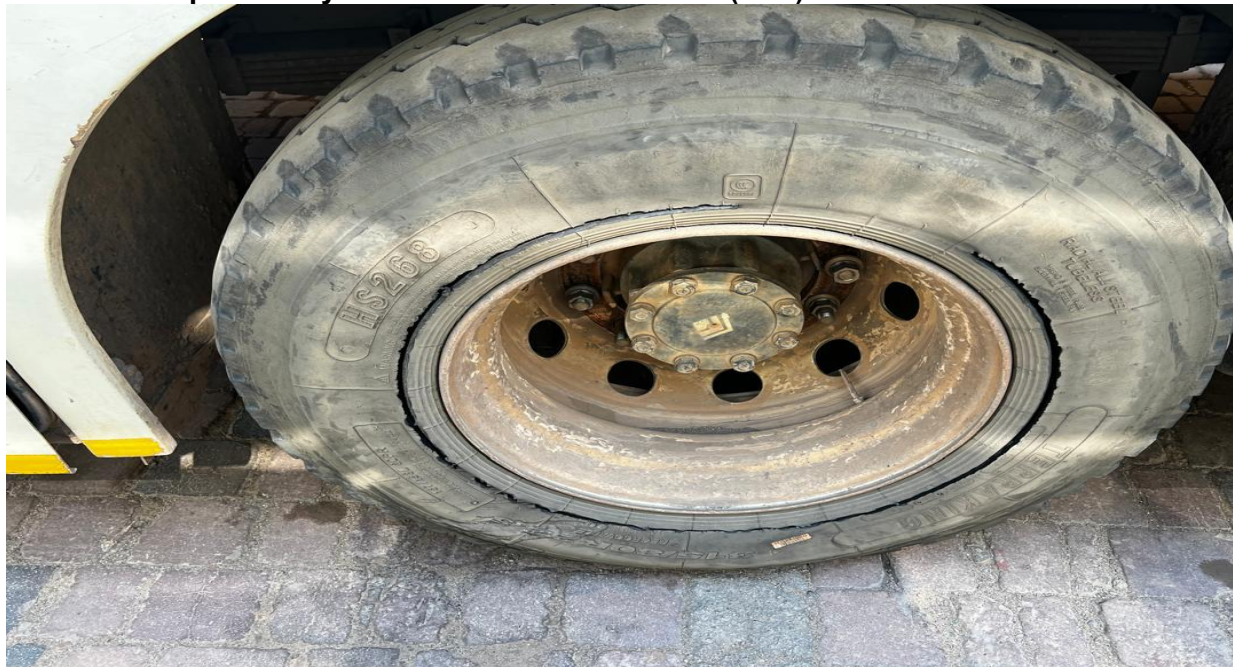
Picture A: Separated Tyre fitted on a ZUPCO-CMED (PVT) LTD Bus 2206.
